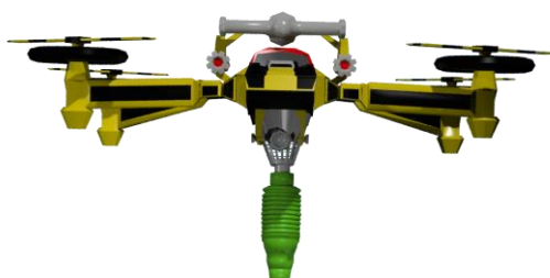
Figure 4. Attaching a VOG 25P ammunition with stabilization to an FPV drone.
